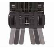
Side Shifter Operators will experience greater efficiency due to fewer required moves when storing and retrieving loads. Integral or hang-on designs available.
