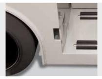
**Battery Gate Interlock Switch** Prevents truck travel if the battery gates are not installed correctly. Operator is notified through an error code on the meter panel.
